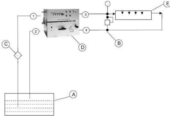
**Fig. 1.** Fuel consumption meter „AVL KMA MOBILE” working scheme [5]:
