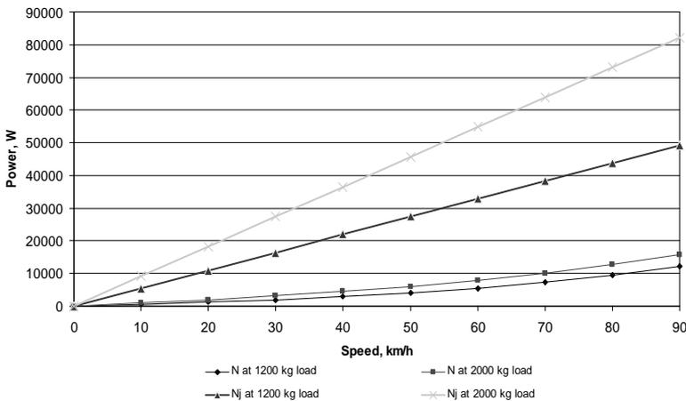
**Fig. 2.** Power to overcome resistances at different load
